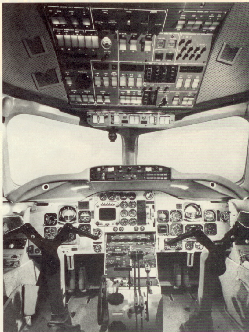
Flight deck has electric, fuel, deicing, air conditioning system and engine start controls on top; nav system selection on the glare shield; flight, power instruments on the panel and avionics grouped on the center console.
